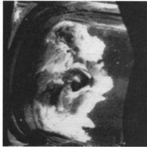
Fig. 6(a) Picture from high speed video under cavitation oscillation component i (for \psi_s = 0.130 \pm 0.002 , \sigma = 0.015 \pm 0.002 )
