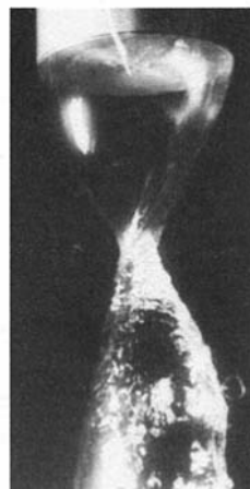
Fig. 3 Multiple tulip formation with swirling effect ( b_o/R_o = 5.71 \cdot 10^{-3} )
