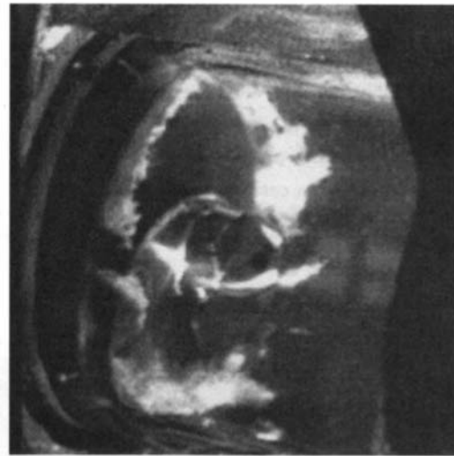
Fig. 6(b) Picture from high speed video under cavitation oscillation component v (for \psi_s = 0.123 \pm 0.002 , \sigma = 0.070 \pm 0.002 )
